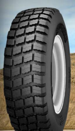
All-steel radial carcass offers puncture resistance and long service life while on hard surfaces
